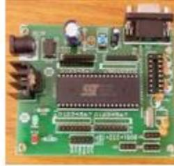
*Fig.2. SST89E516RD2 Microcontroller*
